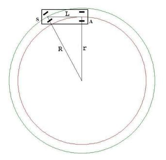
From the above picture, it is obvious, though somewhat surprising perhaps, that the relationship between the two radii R and r and the length L of the vehicle is simply given by Pythagoras theorem, where R and L are known and r is to be calculated:
