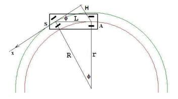
Assume that the front wheels of the vehicle are exiting the traffic circle and are now moving on a straight line. Assume the direction of the x-axis for that straight line. Then V = 0. Hence:
