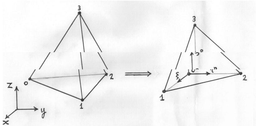
Let's consider the simplest non-trivial finite element shape in 3-D, which is a *tetrahedron*. Function behaviour inside such a tetrahedron is approximated by
