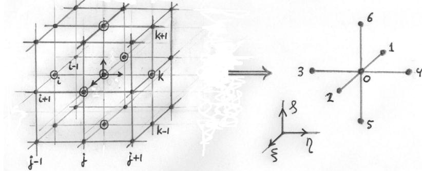
The Finite Difference grid labels ( $i \pm 1, j \pm 1, k \pm 1$ ) are replaced by Finite Element node numbers. Function values ( $T_0, T_1, T_2, T_3, T_4, T_5, T_6$ ) can be defined then at the nodal points. These values can be interpolated by a (Finite Element like) polynomial, which is defined by:
