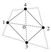
Function behaviour at the sides of a bi-linear quadrilateral is linear.
